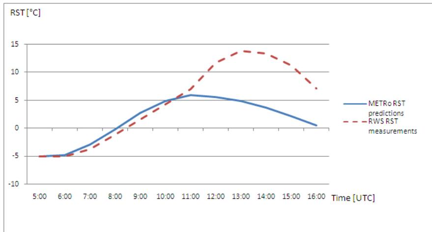
Figure 6. RST predictions calculated at 04:00 and RST measurements at the RWS Šentožbolt on 18 February 2012. RMS error for the RST was  $5.39^{\circ}\text{C}$ .
