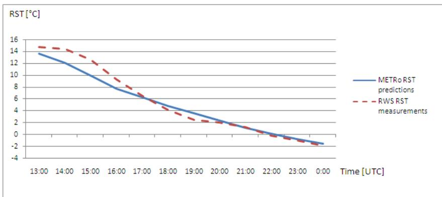
Figure 7. RST predictions calculated at 12:00 and RST measurements at the RWS Sava Šentjakob on 18 February 2012. RMS error for RST was  $1.25^{\circ}\text{C}$ .
