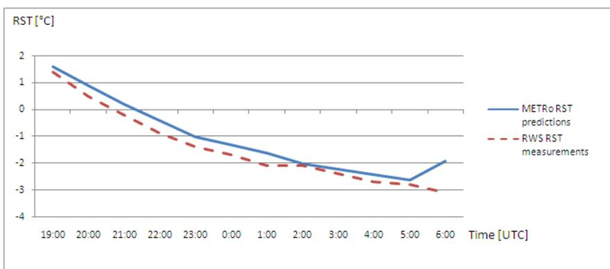
Figure 8. RST predictions calculated at 18:00 and RST measurements at the RWS Slatina on 18 February 2012. RMS error for RST was  $0.48^{\circ}\text{C}$ .
