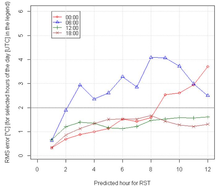
Figure 3. RMS errors for selected hours of the day (roadcasts calculated at 00:00, 06:00, 12:00 and 18:00 UTC) from 1-12 predicted hours for RWS Verd.
